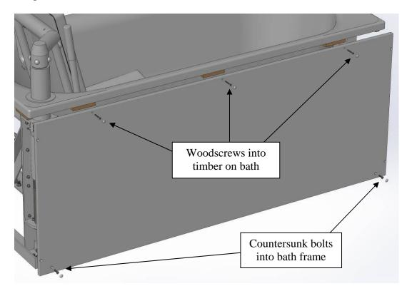
2. With the front panel fitted, the end panel(s) can be fitted. Firstly, these can be secured along one edge to the front panel using M6 x 40 countersunk bolts, which screw through the front panel into the threaded inserts located in the holes in the sides of the end panels. As these bolts are tightened ensure that the end of the front panel is flush with the face of the end panel, and that the top faces are also aligned. The bolts are finished off with a white cap.
