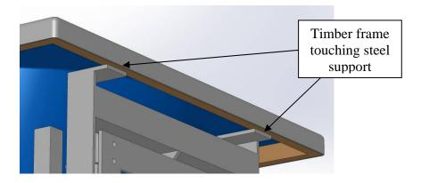
6. Once the bath is sitting down correctly it can be secured in position using the four fixing nuts on the channel supports under the bath.
