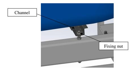
There are 6 grub screws, each located next to one of the fixing points, which can be used to allow for any slight deviations in the floor surface, and also to ensure that the bath is perfectly level. Ideally the frame will be fixed tightly to the surface of the floor, and the grub screws will not be required, but it is important that the frame is not distorted by pulling it against an uneven surface, and the grub screws can be used to take up any gaps which may be present.
